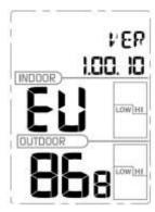
The console will display all of the LCD segments for three seconds after power up, the indoor conditions will immediately update, and the outdoor sensor will register within a few minutes.
